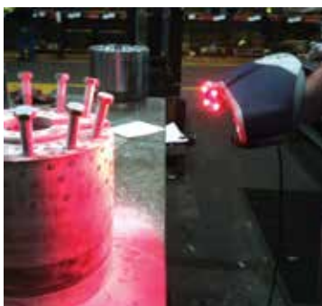
A roll end casing during the 3D laser scanning process. The laser scanner verifies dimensions on finished parts, is used to generate solid models of complex parts, and is a vital part in generating engineering analyses that require high precision and accuracy.
